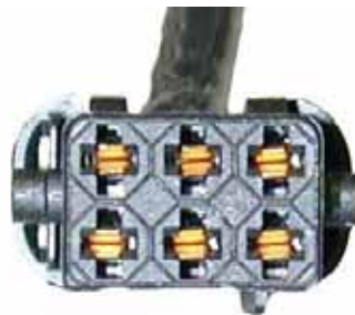
UEGO Sensor connector without latch
