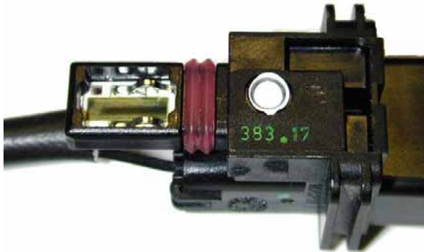
UEGO Sensor laser etched calibration resistor
